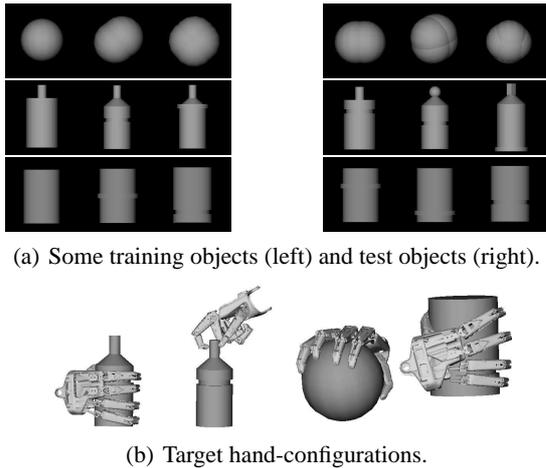
Figure 4: Examples of spherical, cylindrical and bottle objects used to train and test the system, and target hand-configurations.
