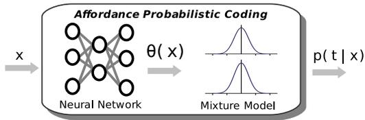
Figure 3: The APC Module is formed by a neural network and a Gaussian mixture model. Given an  $x$  vector, the neural network computes the required Gaussian parameters  $\theta(x)$  to approximate  $p(t|x)$  (see (Bishop, 1995) for more details).
