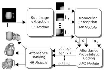
Figure 1: The GA model is formed by four modules: the SE Module, the MP Module, The APC Module, and the AR Module. This computational model receives an image depicting an object as input, and produces a list of affordances (appropriate grasps for the given object) as output.
