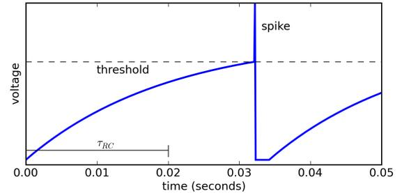
Figure 5: LIF neuron with constant input current.
