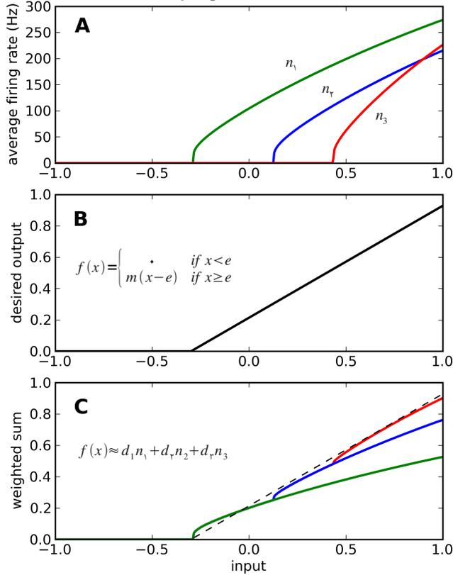
Figure 6: Combining realistic tuning curves to produce a desired function. **A** shows the average firing rate of three different neurons as the amount of input to the neurons increases. **B** shows the neural output function used by the rate neuron model. **C** shows how **B** can be approximated by taking a weighted sum of tuning curves in **A**.
