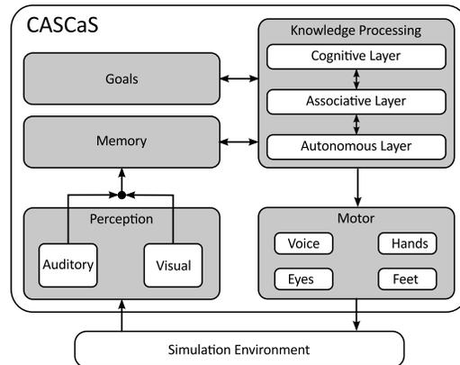
Figure 1: Layered Architecture of CASCaS; (Weber et al., 2013)
