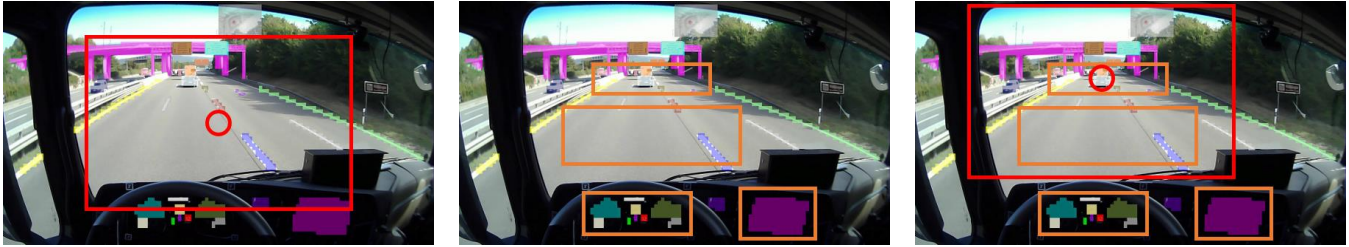
Figure 1: For the module to work, it needs some input data. In this case an annotated camera image. The field of view (red) does not span the entire image. The agent only perceives the color-coded parts, i.e. road surface is invisible to it. The first step is to setup a world simulation and stream data into the ACT-R runtime. The cognitive model manages AoRs (orange). Together they move attention to a car in front (white).
